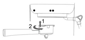
Adjust the filter holder into right direction then insert into machine in " $\bullet$ " location as step 1. Then turn the holder to " $\bullet \bullet$ " location as step 2.
