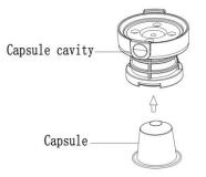
The second step: Put the capsule cavity with capsule into the funnel.
