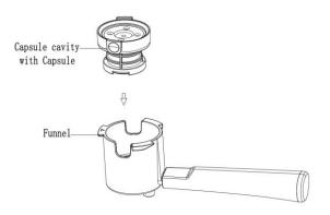
The third step: Install filter holder into machine.
