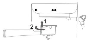
Adjust the filter holder into right direction then insert into machine in " $\bullet$ " location as step 1. Then turn the holder to " $\bullet \bullet$ " location as step 2.
